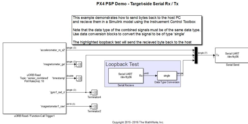
This model is the one that will be deployed the Pixhawk FMU. It will fetch data from a uORB topic and send it off over serial (ttyS6). Loopback data is received and sent back into the serial send block.
