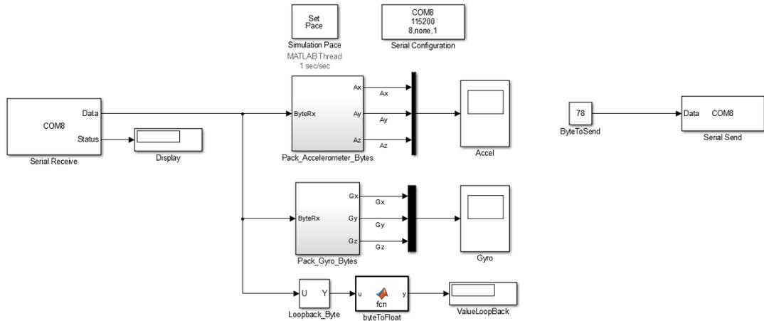
This model does not undergo code generation, it resides on the host PC and is responsible for sending/receiving data to the Pixhawk Px4FMU over serial. The scopes will show accelerometer and gyro readings. A loopback display block is used to show the value that we send to the Pixhawk is sent back.
